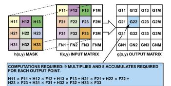
Figure 7. Input matrix, F; 3  $\times$  3 mask matrix, H; and output matrix, G.
