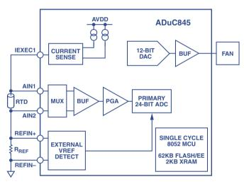
Figure 3. System-on-a-chip implementation.
