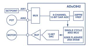
Figure 6. System-on-a-chip implementation of Figure 4.
