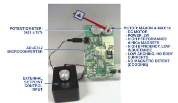
Figure 5. Sample motor control system using discrete components.
