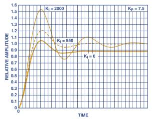
Figure 7. Proportional-integral (P-I) control for three settings of the integral term. Note the offset from 1.0 for  $K_l = 0$ , the lightly damped oscillatory tendency for  $K_l = 2000$ , with oscillations almost eliminated at  $K_l = 550$ .
