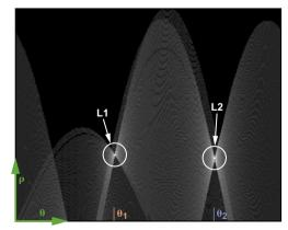
Figure 8c. The Hough transform of the image in Figure 8a. The range for  $\theta$  is  $[0, 2\pi]$ , and the range for  $\rho$  is one-half the diagonal of the input image in Figure 8a. The two bright regions correspond to local maxima, which can be used to reconstruct the two lines in Figure 8a.
