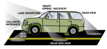
Figure 1. Basic camera-placement regions for automotive safety applications.
