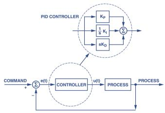
Figure 1. Control loop employing a PID control function.
