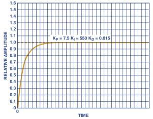
Figure 8. Proportional-integral-derivative (PID) control response.
